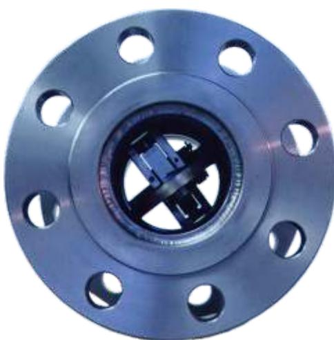
The Breakaway Coupling acts as an identified safe parting point in a hose or loading arm product transfer line, separating in the event of excessive forces being applied, and provides an instantaneous mechanical positive closedown, therefore eliminating from both sides involved, the possibility of human danger, explosion, fire or environmental pollution damage.
